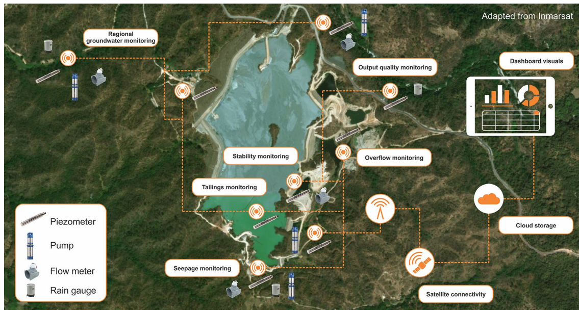
Fig. 12 Location of monitoring points for a typical valley TSF
