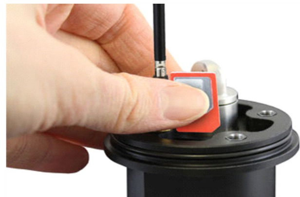
Fig. 7 Wireless transmitter sim card installation
